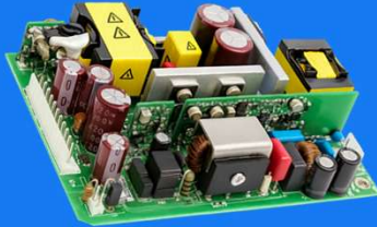
Asymmetrical ZVS Flyback circuit for 300W with PFC
