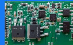
200W Half Bridge LLC Resonant Soft Switching ZVS
