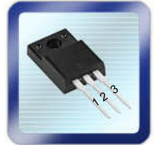
T0220 Full-PAK Isolated (T0-220) 1=Gate, 2=Drain, 3=Source
