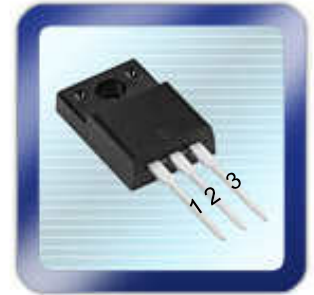
TO220 Full-PAK Isolated (T0-220) 1=Gate, 2=Drain, 3=Source
