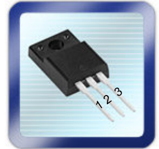
T0220 Full-PAK Isolated (T0-220) 1=Gate, 2=Drain, 3=Source
