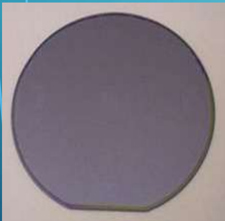
SOI Wafer with <1.5mm edge terrace
