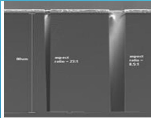
Neighbouring High and Low aspect ratio trenches in SOI without undercut.
